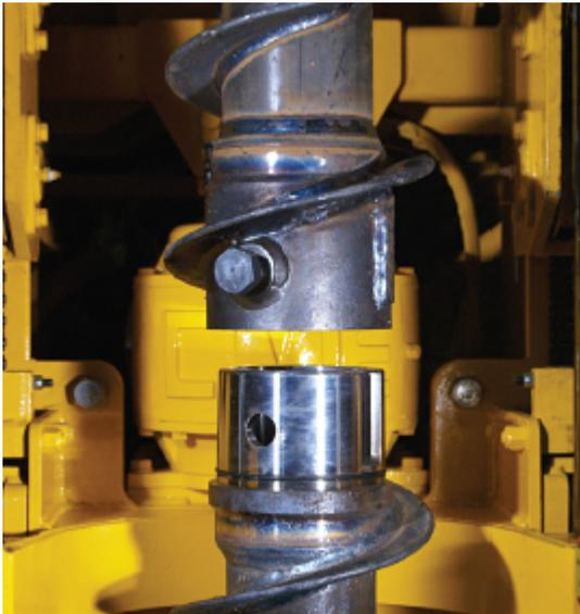
CME augers are able to withstand the torque and retract forces associated with the most difficult drilling conditions. They are designed to be durable, yet relatively lightweight. The auger flighting is the optimum thickness for maximum strength without adding unnecessary extra weight.
