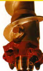
Sampler extended for soft material
