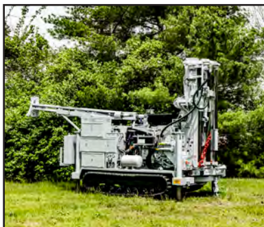
Low Clearance CME-55LCX on CME-300 Carrier
