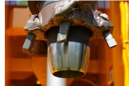
Sampler extended for soft material
