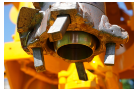
Sampler retracted for more dense material
